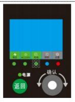
7. Turn the knob to the high voltage icon, press the knob to turn off the high voltage, turn off the light bulb, and enter standby mode.
