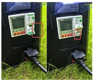
4. Pull out the high-voltage line of the ground power supply, connect it to the airborne power supply as shown in the diagram, and at the same time hook the anti fall hook on the cable into the middle hook of the anti fall steel wire rope.
