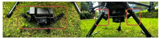
3. Connect the PSDK cable to the EPORT interface at the bottom of the M400, and connect the LP24 interface of the tethered battery to the TE400 airborne battery interface. At this point, the TE400 airborne power supply has been installed.
