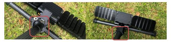
The lighting angle can be adjusted from 0 to 45 degrees.
